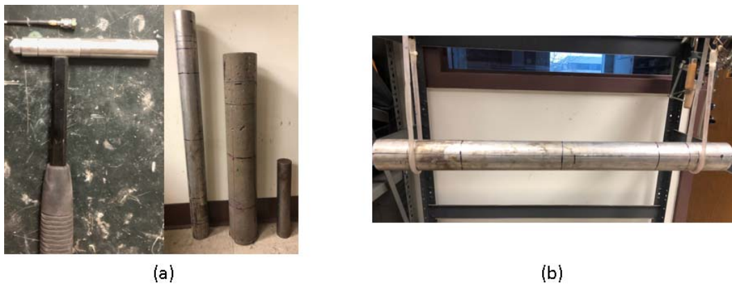
Figure 9. Picture of experiment: (a) Impact hammer, accelerometer, and specimens; (b) Experimental setup.
