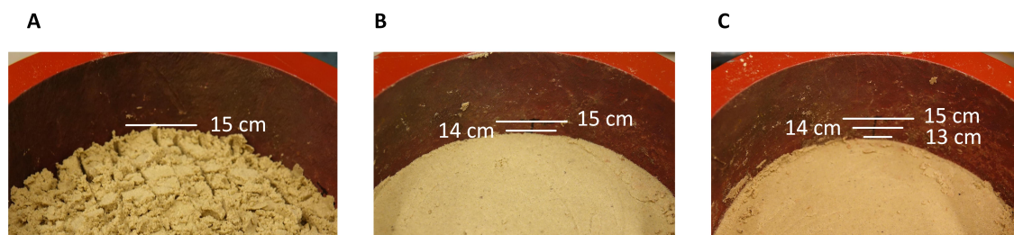
Figure 3. (A) Low traffic condition with the density of 1.35 g/cm 3 . (B) Medium traffic condition with the density of 1.45 g/cm 3 . (C) High traffic condition with the density of 1.55 g/cm 3 .
