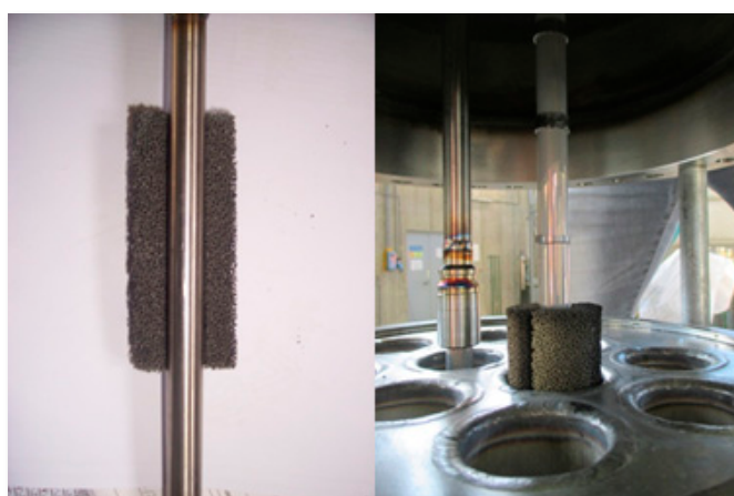
Figure 5. R-02 reactor catalyst arrangement.
