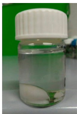
Figure 1. Third phase in the solvent phase after the removal of the aqueous phase for formic acid with 25:25 TOA:1-octanol by weight, diluted in n -undecane; c_{\text{formic, initial}} = 0.8 \text{ mol/L} ; T = 25 \text{ }^\circ\text{C} ; ambient pressure.
