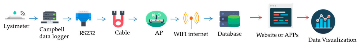
Figure 4. Path of the first version of Information and Communication Technology (ICT) data transmission.
