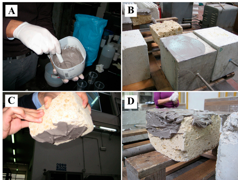
Figure 5. GMK-E composite as soon as obtained by hand mixing (A); and some qualitative test of adhesion and thixotropic behavior on: (B) concrete; and (C,D) tuff. See Ref. [19,27] for details.
