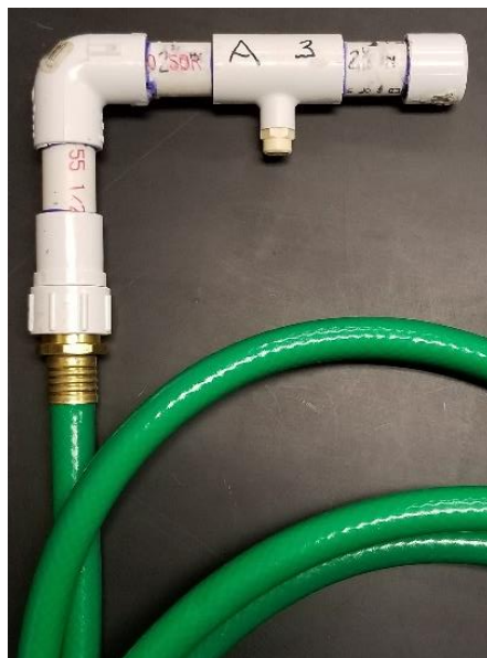
Figure 6. The constructed soil column mister nozzle and piping.
