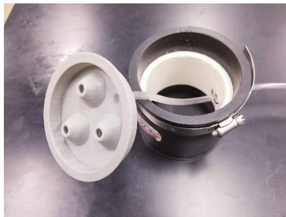
Figure 3. Flow-reduction cap housing. The flow-reduction cap housing consists of the coupling, coupling spacer, flow-reduction cap, and discharge tube. A bead of silicone caulk will be applied around the top of the coupling spacer that touches the lip of the flow-reduction cap.
