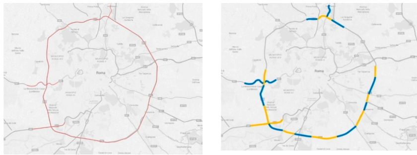
Figure 4. Basic noise maps preparation: split the road network in arcs corresponding to the elementary noise sources.
