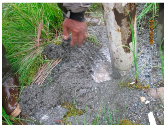
Figure 6. Sample collection at DDH 7382. Material collected at base of drill stem had a gravel texture, but putty-like texture as gravel was scooped away
