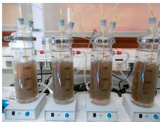
Figure 2. Organization for Economic Co-operation and Development (OECD) test for the biodegradation of a fire-fighting foam containing a polyfluoroalkyl ether.
