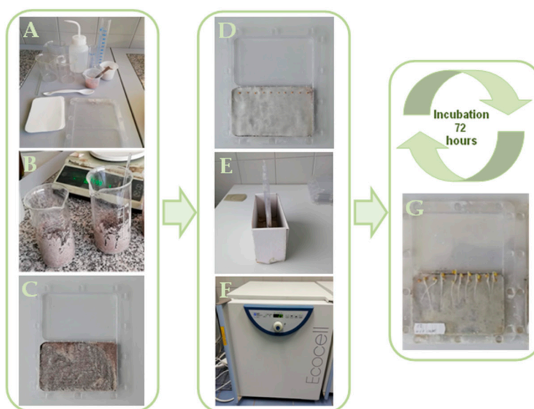
Figure 2. Process of test phytotoxicity of leachate. Images of (A) preparation of laboratory instruments, (B) mixture of OECD soils with a blank sample, (C) application of the mixture to the sample box, (D) application of Sinapis alba L. seeds, (E) closing and placing the sample box in the holder, (F) incubation of the mixture in Ecocell oven, (G) evaluation.
