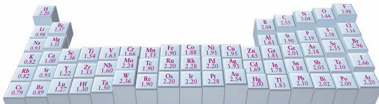
FIGURE 3.7 Average electronegativity of atoms, computed with the method that Linus Pauling developed. Electronegativity values have no units.
