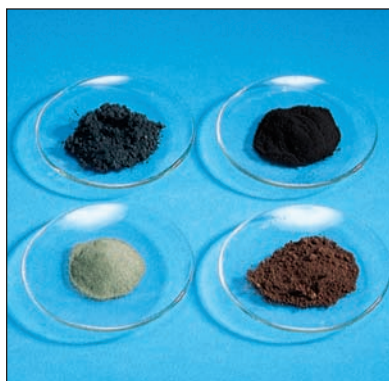
FIGURE 3.23 Several oxides of manganese. They are arranged in order of increasing oxidation number of the Mn, counterclockwise from the bottom left: MnO, Mn 3 O 4 , Mn 2 O 3 and MnO 2 . A compound of still higher oxidation state, Mn 2 O 7 , is a dark red liquid that explodes easily.
