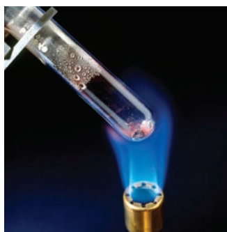
FIGURE 1.6 When the red solid mercury(II) oxide is heated, it decomposes to mercury and oxygen. Note the drops of liquid mercury condensing on the side of the test tube.
