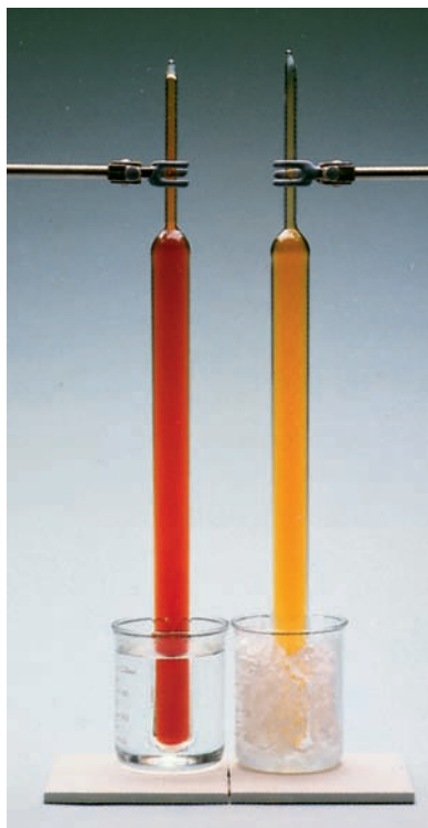
FIGURE 14.9 The equilibrium between \text{N}_2\text{O}_4 and \text{NO}_2 depends on temperature. The tube on the right, held in an ice bath at 0^\circ\text{C} , contains mostly \text{N}_2\text{O}_4 . Its color is pale because only \text{NO}_2 is colored. The deeper color in the tube on the left, which is held at 50^\circ\text{C} , reflects the increased \text{NO}_2 present in equilibrium at the higher temperature. The tubes contain the same masses of substance, distributed in different ways between \text{NO}_2 and \text{N}_2\text{O}_4 .
