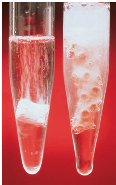
FIGURE 9.1 The calcium carbonate in a piece of chalk reacts with an aqueous solution of hydrochloric acid to produce bubbles of carbon dioxide.
