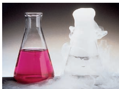
FIGURE 15.15 The indicator phenolphthalein is pink in basic solution ( left ). When dry ice (solid carbon dioxide) is placed in the bottom of the beaker ( right ), it dissolves to form carbonic acid. This neutralizes the base in solution, and causes the indicator to change to its colorless form characteristic of an acid solution.
