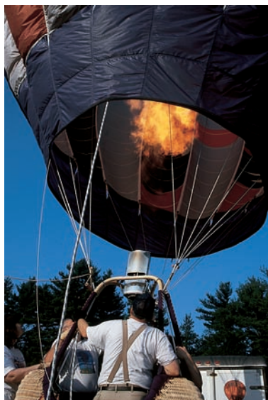
FIGURE 9.7 In a hot-air balloon, the volume remains nearly constant (the balloon is rigid) and the pressure is nearly constant as well (unless the balloon rises very high). Thus, n is inversely proportional to T ; as the air inside the balloon is heated, its amount decreases and its density falls. This reduced density gives the balloon its lift.
