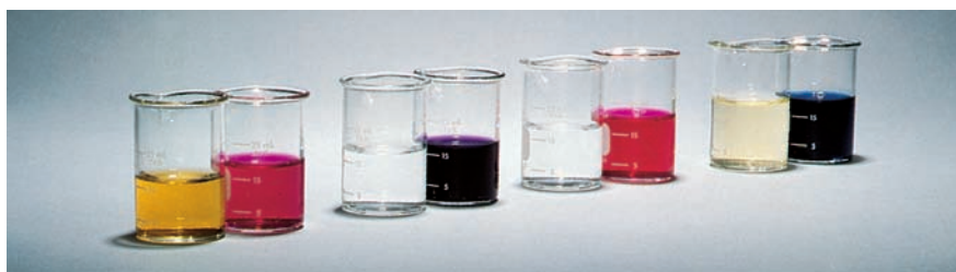
FIGURE 15.8 Color differences in four indicators: bromophenol red, thymolphthalein, phenolphthalein, and bromocresol green. In each case the acidic form is on the left and the basic form is on the right.
