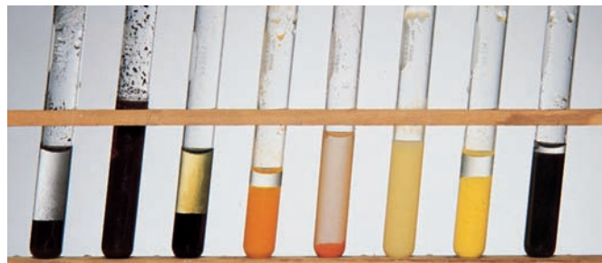
FIGURE 16.10 These sulfides are insoluble at pH 1, so they can be separated out of a mixture containing other, more soluble sulfides. From left to right, they are PbS, Bi 2 S 3 , CuS, CdS, Sb 2 S 3 , SnS 2 , As 2 S 3 , and HgS.
