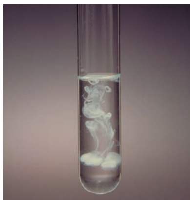
FIGURE 11.5 A solution of potassium sulfate is being added to one of barium chloride. A cloud of white solid barium sulfate is formed; the potassium chloride remains in solution.
