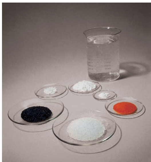
FIGURE 16.2 Vastly different quantities of different compounds will dissolve in 1 L of water at 20°C. Clockwise from the front are borax, potassium permanganate, lead(II) chloride, sodium phosphate decahydrate, calcium oxide, and potassium dichromate.
