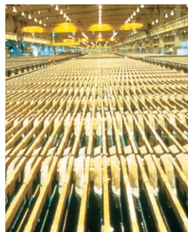
FIGURE 17.18 In the electrolytic refining of copper, many slabs of impure copper, which serve as anodes, alternate with thin sheets of pure copper (the cathodes). Both are dipped into a dilute acidic solution of copper. As the copper is oxidized from the impure anodes, it enters the solution as \text{Cu}^{2+} and migrates to the cathodes, where it plates out in purer form.
