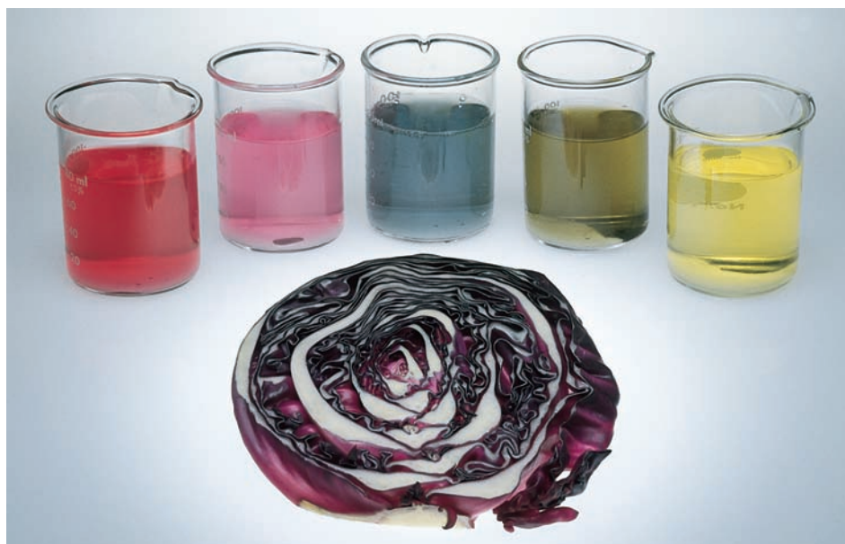
FIGURE 15.10 Red cabbage extract is a natural pH indicator. When the solution is highly acidic, the extract gives the solution a red color. As the solution becomes less and less acidic (more basic), the color changes from red to violet to yellow.
