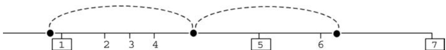
Figure 4.10 A systematic unequal probability sample of size 3 from a population of size 7.
