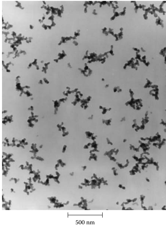
FIGURE 14.1 Soot fractal aggregates with fractal dimension D_f = 1.78 \pm 0.07 .
