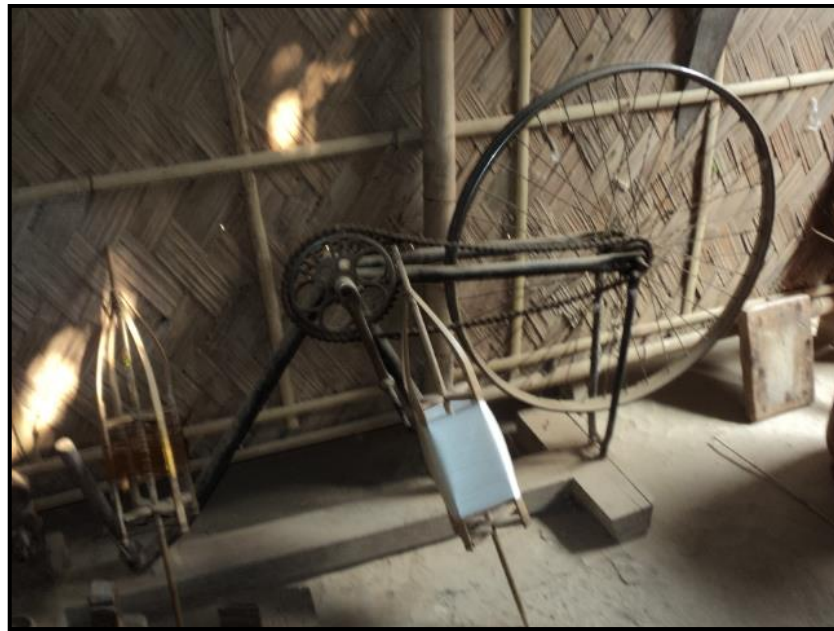
Plate 3.4: Instrument which is used for reeling of the yarn from the cocoons
