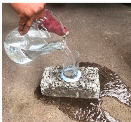
Figure 3. Infiltration rate test.
