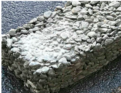
Figure 6. Pervious concrete with 25% recycled rubber aggregates after being cured.
