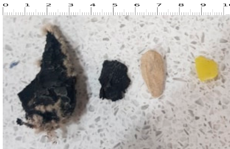
Figure 1. Recycled tire rubber, crushed dolomite, and waste plastic aggregates.
