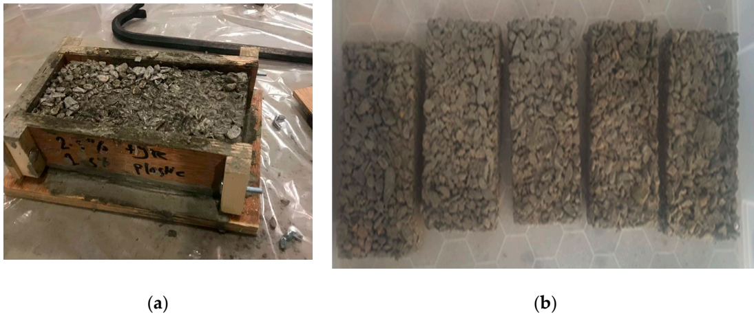
Figure 2. (a) Hardened sample before being demoulded. (b) Curing samples in water.
